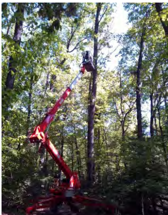
RA Arborist using a spider-lift to prune trees. Photo courtesy of Claudia Thompson-Deahl
